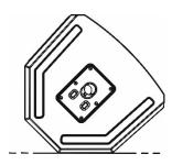
The rear side inclination, symmetrical, as shown in the upper picture, is 40°. SYA10 can be used as a stage monitor in small contexts, in this case please consider the characteristic dispersion pattern presented above.
