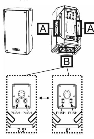
A – Lateral integrated handles B – Pole mount hole, with two tilt angles selection (0°/ 7.5°)
