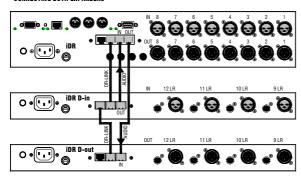
Fully expanded iDR-4(8) The diagram below shows the iDR-8 with both the input and output digital expanders fitted. Note the connection of DR-Link which is daisy chained from one unit to the next. If an iDR-switch unit is also fitted then daisy chain DR-Link from the last expander to the switch unit. Make sure you plug into the correct DR-Link socket.
