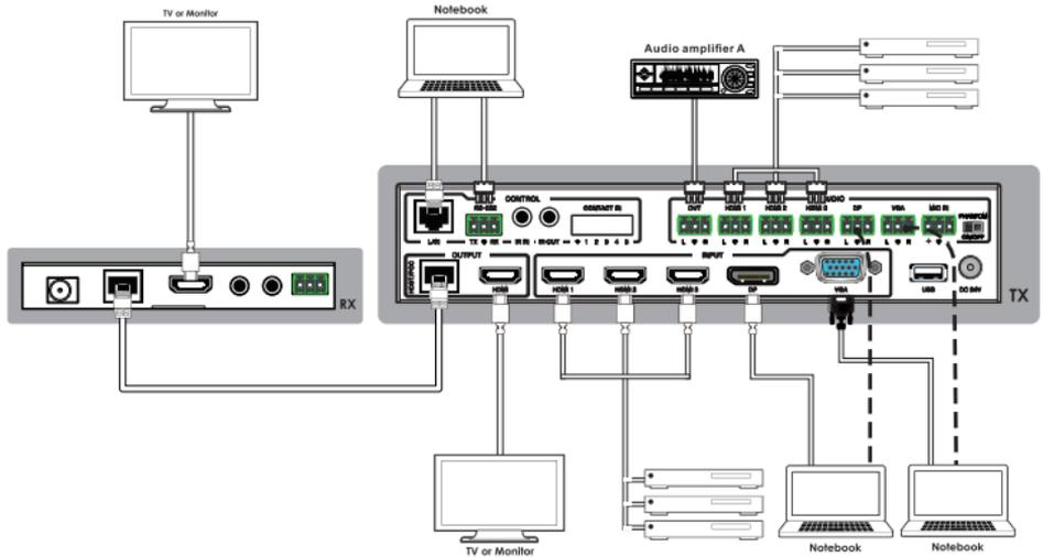
1. Connect HDMI source devices (e.g. Blue-ray DVD) to HDMI input ports of the switcher with HDMI cable. Connect VGA source device (eg.PC/Note-book) to VGA input port of the switcher with a VGA cable.
