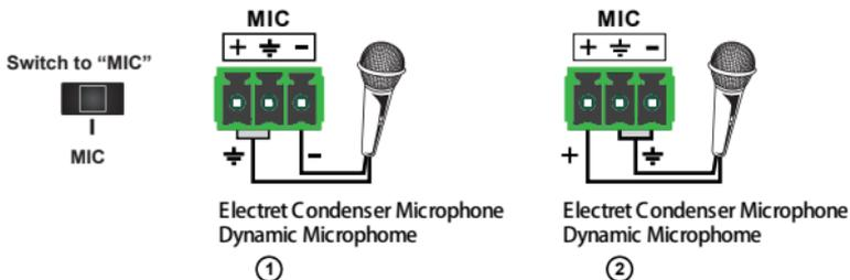
2) **Balanced connection:** “+” connects to positive, “-” connects to negative and “ $\frac{\pm}{\text{g}}$ ” connects to ground.
