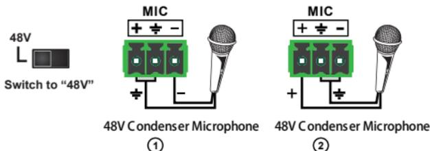
**2) Balanced Connections:** "+" connects to positive, "-" connects to negative and "GND" to ground.
