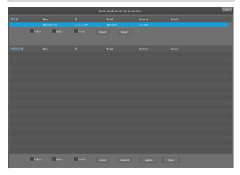
After selecting the same model of the device to be synchronized that is currently managed and unchecked, tick any or more of the video parameters, audio parameters, and trace parameters, and when you click the sync parameters, the device that you are currently synchronizing will synchronize with the source device parameters.
