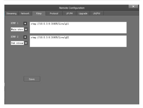
In RTMP1 and RTMP2, main stream, sub stream can be chosen to stream.
