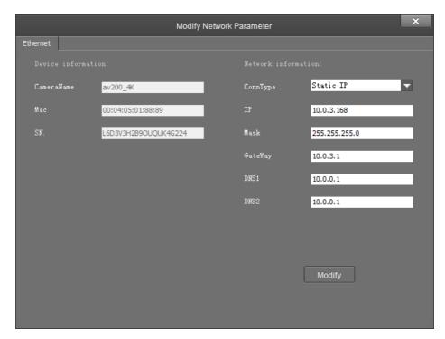
To control and preview a camera, first choose the device, modify its IP address as the IP address of the same LAN, then click "Add to Client" as the picture shown below.
