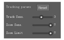
**Tracking Sens:** Set sensitivity of tracking enable to detect and track. High sensitivity easily, and not lose the object.
