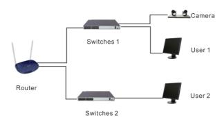
Please refer to the above diagram, userl and user 2 are in the same router, they are considered as in the same LAN, connect the camera to the same LAN as where the PC is, and refer to below instructions as how to use the application software, then the camera can be found and connected from the online device list.
