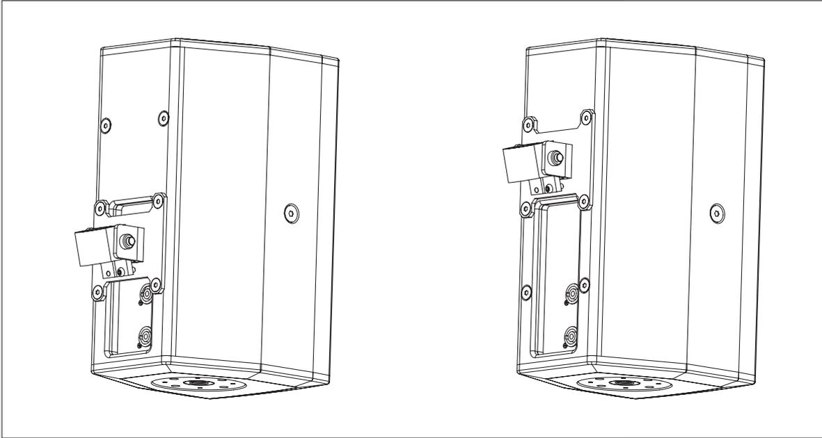
Add the two included bars to mount the swivel bracket at the centre (allowing also a balanced horizontal mounting of the loudspeaker).
