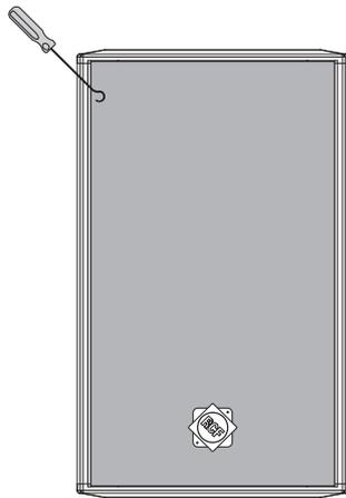
Using a hook, pass through the foam layer and try to locate a hole on a side of the metal grille
