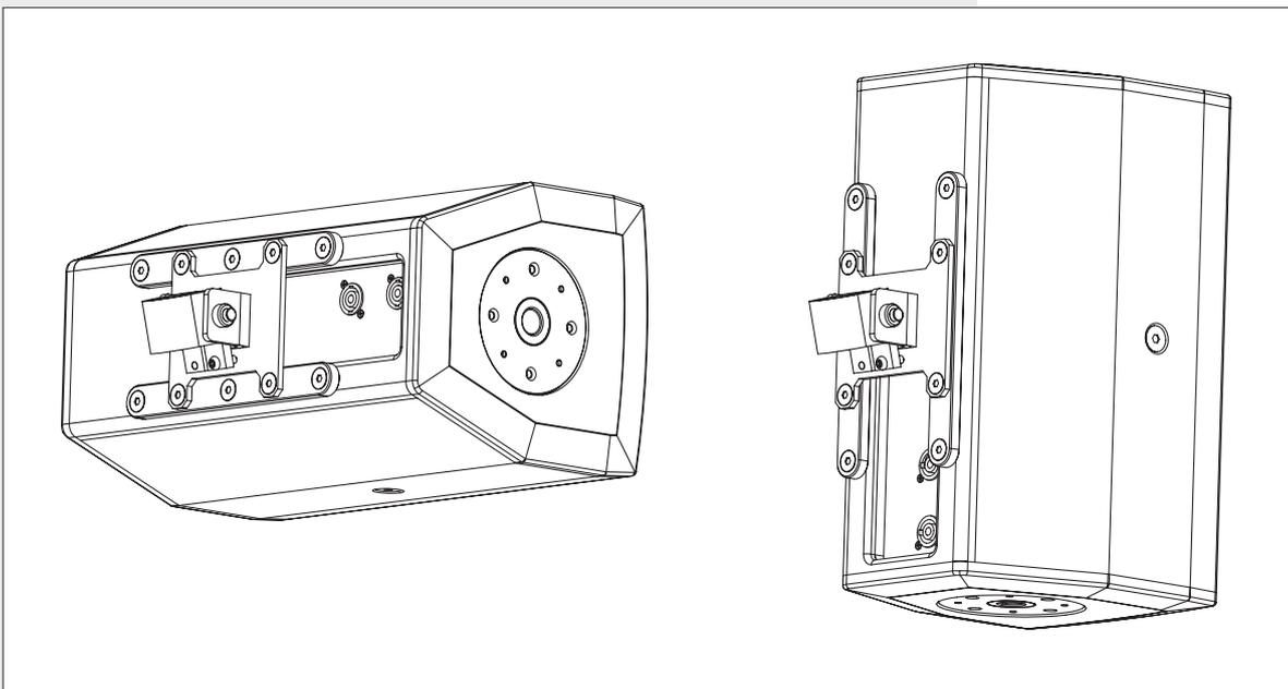
The C3110 models have 8 threaded holes (instead of 6), allowing the direct mounting (without additional bars) of the AC WM-C accessory at the rear panel centre.
