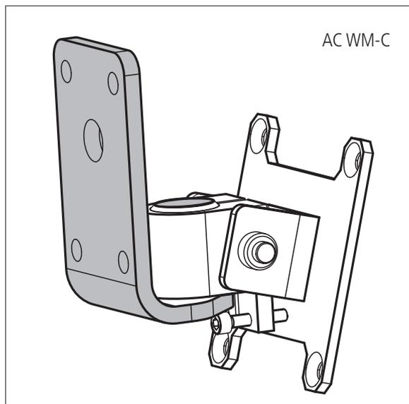
About the C3108 models, it is possible to fix the moving part of the AC WM-C accessory directly to the loudspeaker rear panel, through four M8 flat head screws, in one of the 2 possible positions.
