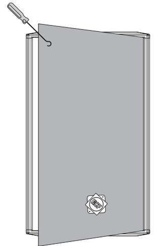
Once the hook is hanged to the metal grille, pull gently. The grille should now lift and can be removed
