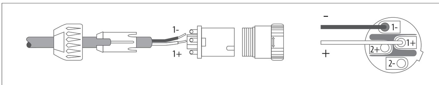
Connect the positive wire (amplifier '+' output) to the pin 1+ of the SPEAKON connector.
