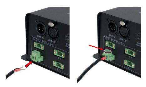
Now insert the wire leads from the fixture into the wire terminals of the Phoenix connector, making sure that the bare wire lead ends have been fitted with wire end sheaths. Tighten the two screws above the wire terminals, as shown in the image at above right, to secure the wire leads in the Phoenix connector.
