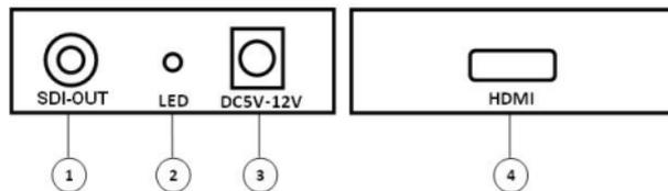
**SDI-OUT:** This slot is where you connect the SDI display with coaxial cable .
