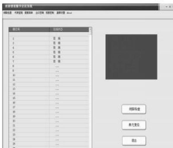
Click to enter the "Line Check" window, click the "Line Check" button to detect all the units of the system. If the unit status is normal, "Online" will be displayed.
