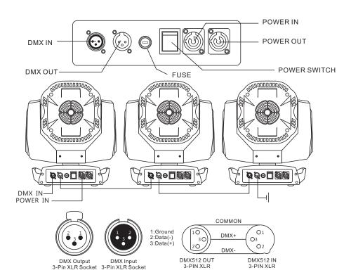
For installations where the DMX cable has to run a long distance or is in an electrically noisy environment, such as in a discotheque, it is recommended to use a DMX terminator. This helps in preventing corruption of the digital control signal by electrical noise. The DMX terminator is simply an XLR plug with a 120  $\Omega$  resistor connected between pins 2 and 3,which is then plugged into the output XLR socket of the last fixture in the chain. Please see illustrations below.
