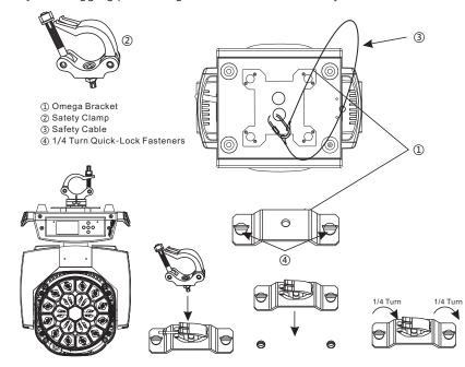
Regardless of the rigging option you choose for your JNR MANTIS 1915, always be sure to secure your fixture with a safety cable. The fixture provides a built-in rigging point for a safety cable on the hanging bracket as illustrated above. Be sure to only use the designated rigging point for the safety cable and never secure a safety cable to a carrying handle.
