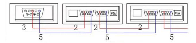
If using signal amplifier, us the wire of RS232 to connect signal amplifier, then use amplifier to connect with each unit lift, just like parallel connection.
