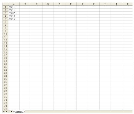
Note:In this data file,the numbers in column A,row 1 is 29,11 means bank29,scene 11.Row1-row5 is 29+11;26+11;29+07;26+13;26+15 means that when you run the chase 1 in the cotroller,run order is bank29,scene11→bank26,scene11 →bank29,scene07→bank26,scene13→bank26,scene15 in loop which stored SD-card.
