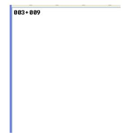
Note:In this data file,the number 003 means you have set the Pan axis channel address to 3;the number 009 means you have set the Tilt axis channel address to 9.
