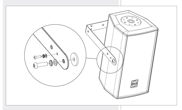
As an alternative, it is possible to install the loudspeaker a bit less prominent, tanks to the U bracket inner holes.
