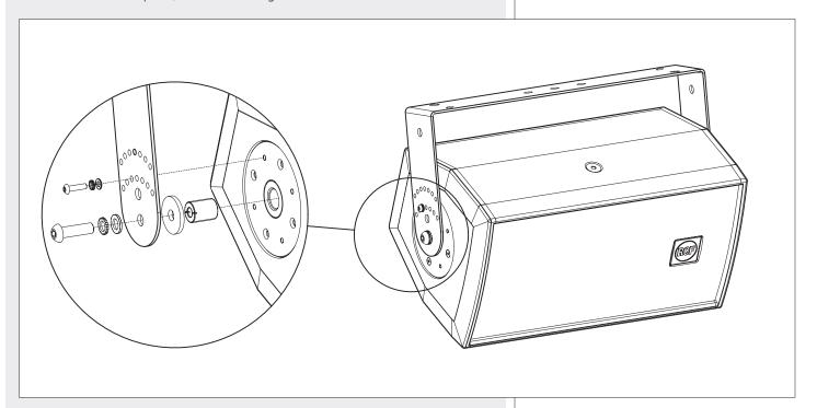
As an alternative, it is possible to install the loudspeaker a bit less prominent, tanks to the U bracket inner holes. Before tightening the two M10 bolts, adjust the loudspeaker vertical tilt and then fix it through two M5x20 bolts into one of the 7 small holes of the U bracket.
