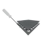
Notice the metal grille is located under a foam layer. THE HOOK MUST BE HANGED TO THE METAL GRILLE. DO NOT PULL IF THE HOOK IS HANGED TO THE FOAM LAYER.
