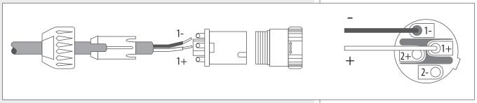
Connect the positive wire (amplifier '+' output) to the pin 1+ of the SPEAKON connector. Connect the negative wire (amplifier '-' output) to the pin 1- of the SPEAKON connector. The pins 2+ and 2- are not used.
