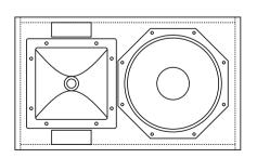
rotate HF horn 90° for horizontal orientation
