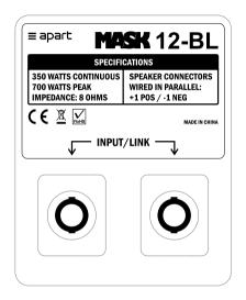
Input: the signal from a power amplifier must be connected to the input/link speakon® connector. The connectors are equivalent and internally wired in parallel. Connector 1+ (positive) and 1- (negative) are used. 2+ and 2- are not connected.
