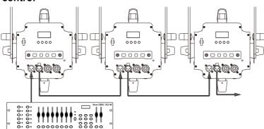
A DMX512 data link is required in order to control the device via DMX. The device provides 3-pin XLR connectors for DMX connection.
