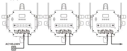
The device uses an auto-range power supply that accepts input voltages between 100 und 240 volts.
