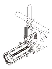
For use on a lighting stand, place the device on a lighting stand via the TV spigot and fasten the fixation screw. Suitable stands can be found in the "Accessories" section
