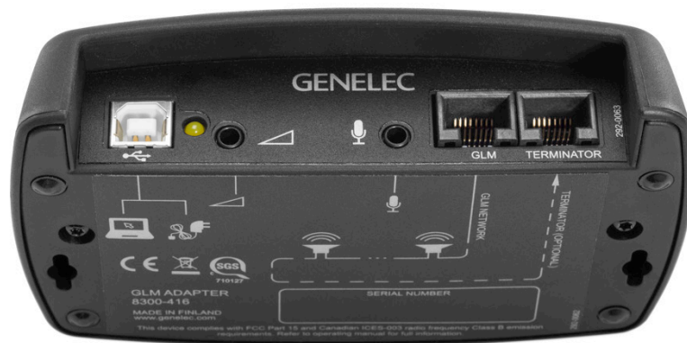
Figure 31. GLM Network Adapter connections from left to right, USB to computer or to USB power supply, hardware level controller input, GLM measurement microphone input, GLM network and terminator connectors.
