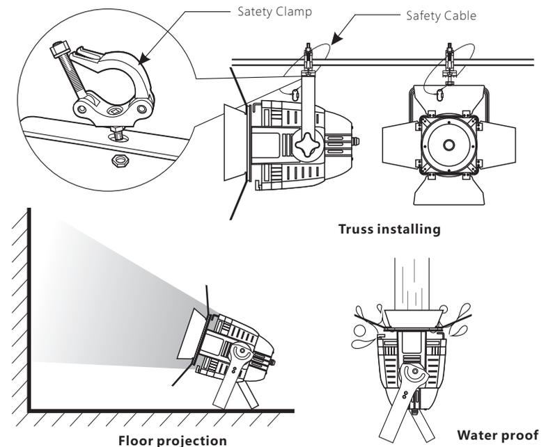
Regardless of the rigging option you choose for your PAR LED COB 200CWWW, always be sure to secure your fixture with a safety cable. The fixture provides a built-in rigging point for a safety cable on the hanging bracket as illustrated above. Be sure to only use the designated rigging point for the safety cable and never secure a safety cable to a carrying handle.
