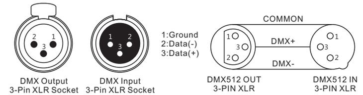
For installations where the DMX cable has to run a long distance or is in an electrically noisy environment, such as in a discotheque, it is recommended to use a DMX terminator. This helps in preventing corruption of the digital control signal by electrical noise. The DMX terminator is simply an XLR plug with a 120  $\Omega$  resistor connected between pins 2 and 3, which is then plugged into the output XLR socket of the last fixture in the chain. Please see illustrations below.
