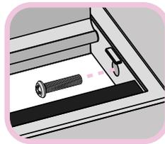
Once the screw touches the edge, begin fastening the second screw until it touches the other edge. **Don't fasten it further than that.**
