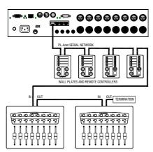
**PL-Anet** is the proprietary Allen & Heath system for daisy chaining remote controllers. It is an RS485 serial connection that uses CAT5 STP cable to communicate between devices over long distances. It requires a terminator at the last unit in the chain. PL-Anet only works with Allen & Heath **PL** devices. The connection includes +20V DC to power the connected devices. The **iDR-8** port is shown here.
