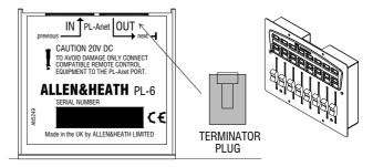
**End of chain termination** As with any RS485 system, the last **PL** device needs to have a terminating resistor fitted to its output port. The **PL-6** is shipped with an RJ45 terminator plug with this resistor built in. Plug the terminator into the last unit in the PL-Anet chain. If the **PL-6** is the only unit connected make sure the terminator is plugged into its output port.
