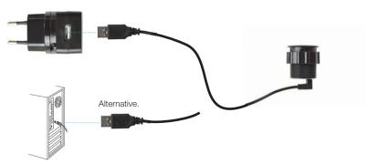
PM30(W) has a small power adapter included. You can also connect the USB cable to any other USB port.
