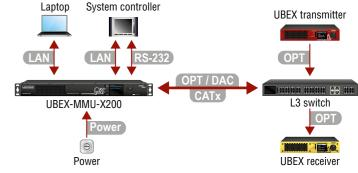
CONNECT the MMU and the L3 network switch by an optical cable or DAC cable (via the SFP slot), or CATx cable (via the CATx connector).
