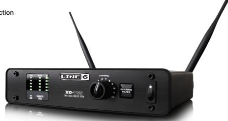
The XD-V55L digital wireless lavalier microphone system sets a new audio quality standard in lavalier systems for spoken word performers and musicians. With 12 channels of 24-bit, 10Hz–20kHz, compander-free performance, the XD-V55L provides unmatched full-range audio clarity and license-free operation worldwide.
