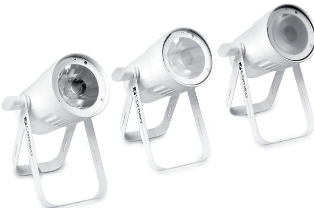
**EN** Two diffuser screens with a different beam dispersion ( $1 \times 10^\circ$ ,  $1 \times 25^\circ$ ) are supplied with the spot. The beam angle of the spotlight can thus be adjusted individually to  $4.5^\circ$  (without diffuser), or  $25^\circ$ . Set the desired diffuser screen in front of the light-emitting lens and secure it with the help of the supplied safety ring.
