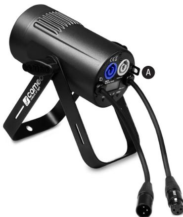
**EN** Thanks to the integrated double bracket, the spotlight can be placed in a suitable location on a flat surface. Mounting on a truss is performed with the help of a suitable truss clamp (not included). Make sure that the connection to the mounting bracket is solid, and secure the device with a suitable safety rope to the space provided (A). Important Notice: Overhead installation should only be carried out by trained personnel.
