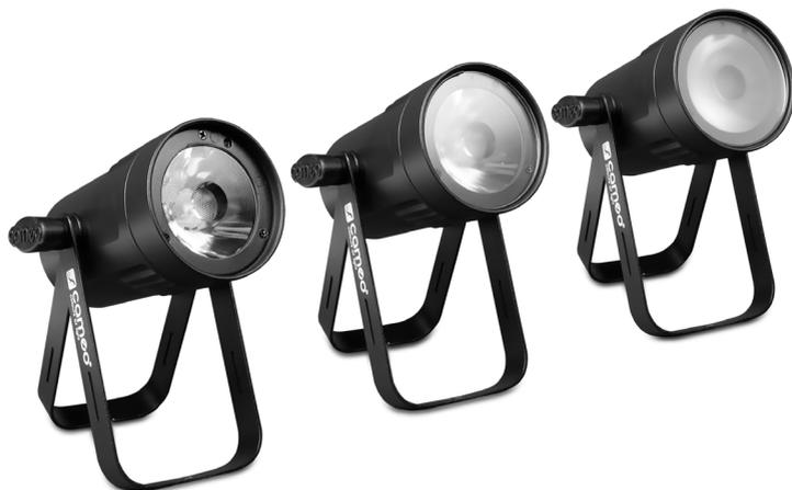
**EN** Two diffuser screens with a different beam dispersion (1 x 10°, 1 x 25°) are supplied with the spot. The beam angle of the spotlight can thus be adjusted individually to 4.5° (without diffuser), or 25°. Set the desired diffuser screen in front of the light-emitting lens and secure it with the help of the supplied safety ring.
